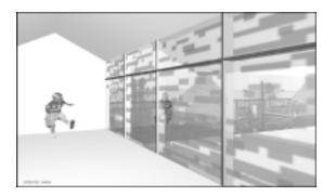
justs its transparency to compensate for changing outside light-levels. It was also part of the intension that through the incorporation of touch sensors users could interact directly with the wall, for instance "drawing" a window where they need light or a view. This chameleon-like construction adjusts its skin in response to changes in the weather or the moods of its users.
